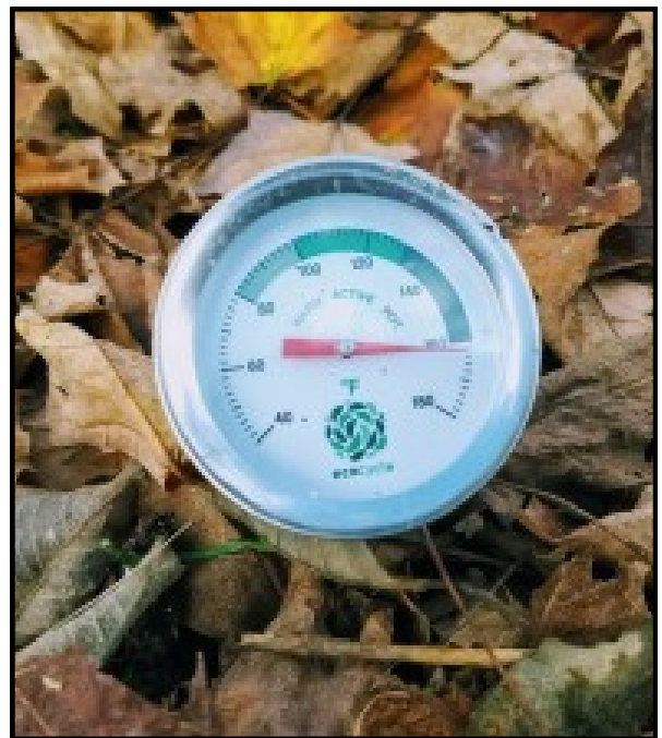
A long-stemmed thermometer can take the temperature at the center of a compost pile
